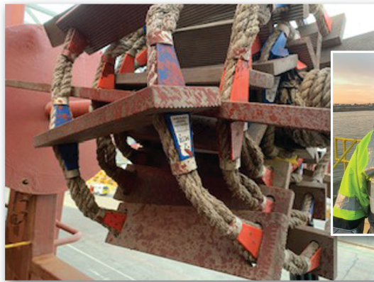
Ladder liberally splattered with 'red lead' paint which should have immediately condemned it.
