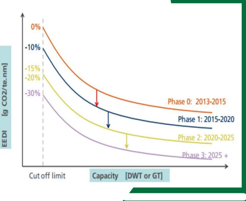
The reduction factor is used to tighten the EEDI regulations in phases over time by increasing its value so that the ship's engines are getting more energy efficient. Required EEDI = (1 - x/100) x Reference line value where x = Reduction factor
