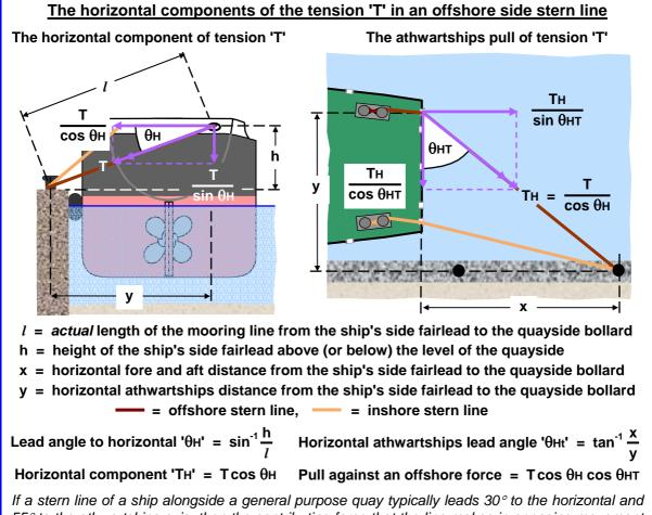
If a stern line of a ship alongside a general purpose quay typically leads 30° to the horizontal and 55° to the athwartships axis, then the contributing force that the line makes in opposing movement off the berth is given as:-
