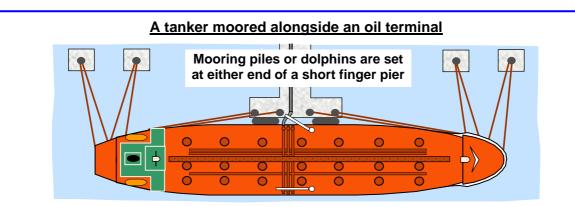
The tanker is held alongside by long breast lines running out from the bow and the stern to bollards on the dolphins whilst springs hold the ship in the correct fore and aft position.
