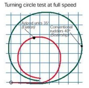
On a theoretical point of view, the azipod should offer a bigger dynamism in the control of the command and also reduced turning circles. These characteristics drive the builders to point out the reduced times for handling but also the consumption reductions and the high swinging abilities.
