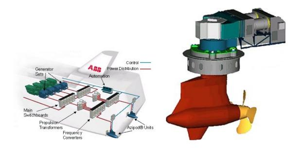
The pod principle is set in an electrical engine fitted in a hub that can be orientated over  $360^{\circ}$ . This engine is coupled to a shaft as short as possible on which is connected a reversible propeller. The electrical variation of rotation speed allows a very thin control of the shaft speed, very smooth, with a big torque since the reduced speeds very close to the zero rotation. The azipod maximum power is close to 25 MW.
