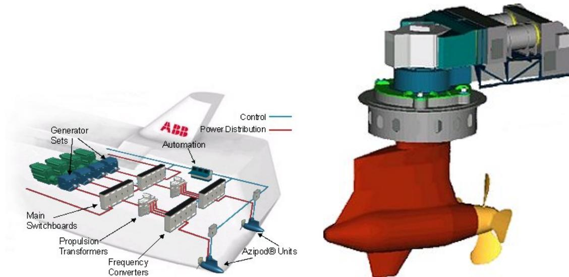
The pod principle is set in an electrical engine fitted in a hub that can be orientated over 360°. This engine is coupled to a shaft as short as possible on which is connected a reversible propeller. The electrical variation of rotation speed allows a very thin control of the shaft speed, very smooth, with a big torque since the reduced speeds very close to the zero rotation. The azipod maximum power is close to 25 MW.
