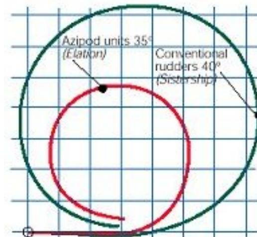
On a theoretical point of view, the azipod should offer a bigger dynamism in the control of the command and also reduced turning circles. These characteristics drive the builders to point out the reduced times for handling but also the consumption reductions and the high swinging abilities.
